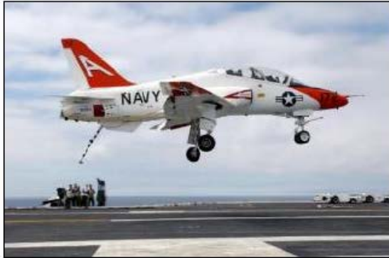
Trainer Jet Ferrium M54 steel hookshank
