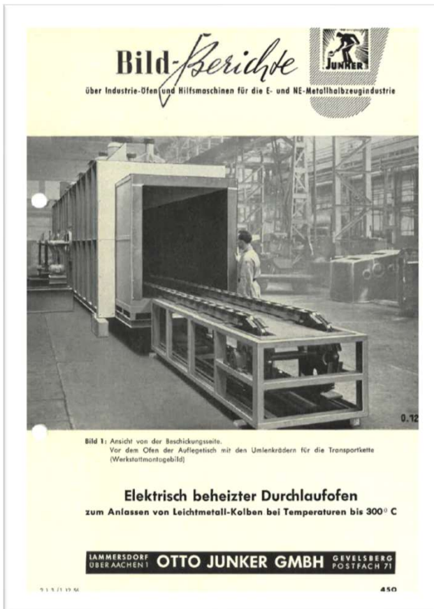
Electrical heated continuous furnace / example of a furnace flyer of 1956
