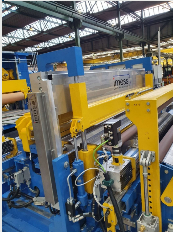
Installation between roll cage and felt brake
